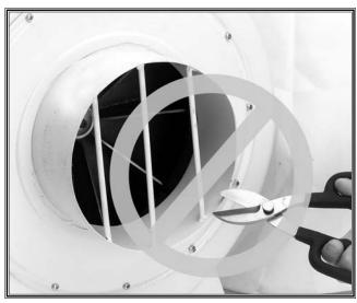
Figure 5. Do Not remove impeller guard.
